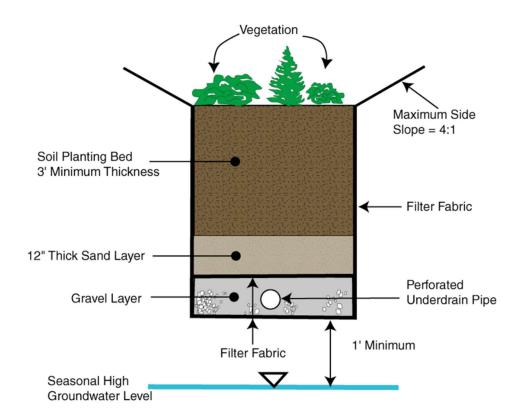
**Typical Bioretention Section Detail**
